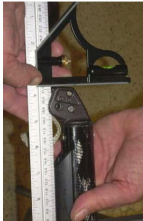
Top and heel points: In many cases, the heel point is also the mast datum point.
