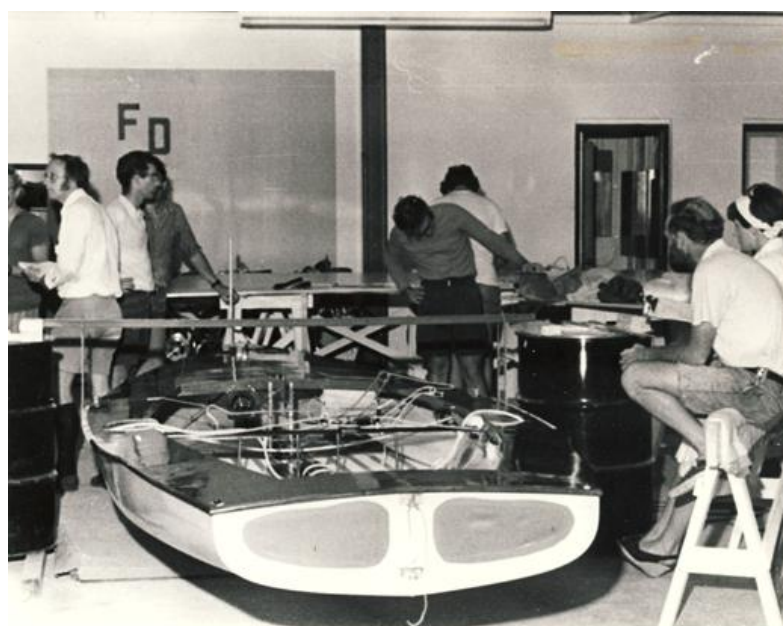
Figure H.4.1.4 An FD undergoing a Lamboley test at the 1976 Olympics, as demonstrated to Queen Elizabeth.
