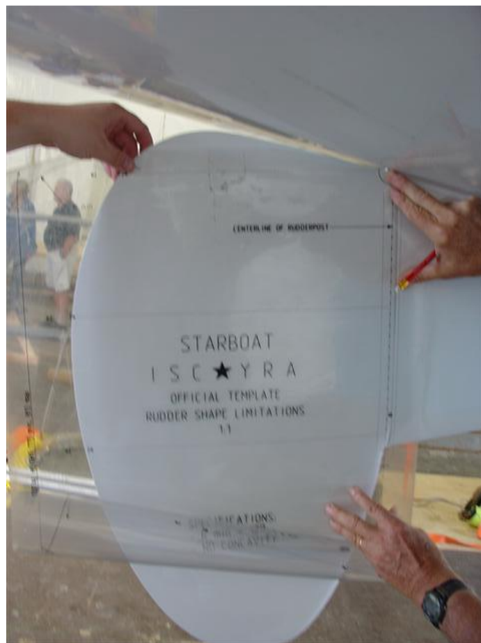
Figure I.5.4 Profile check with mylar template.
