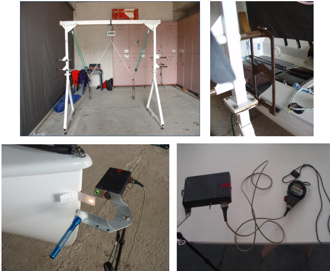
Figure H.4.2.1 A modern Finn Lamboley system showing the pairs of retractable knife edges, the Finn hooks with bearings 200 mm apart and the photocell used for timing.
