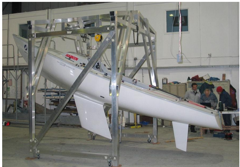
Figure H.4.7.2 The 2004 tilt swing system installed on the keel bolts of an Yngling. The swing bearing is mounted on a precision rail and the position read on the electronic scale. The box below the “rail scale” is the inclinometer. The roller bearing and the shackles for the support and steady lines of the suspension can be seen at the top of the photograph.
