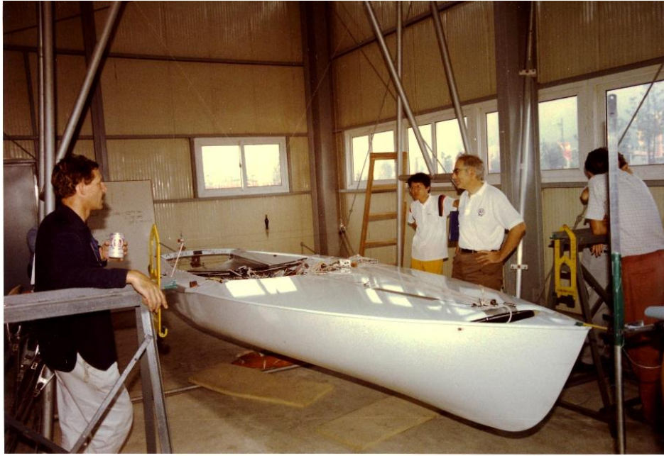
Figure H.4.8.2 A Flying Dutchman on a bifilar suspension at the 1988 Olympics in Pusan. Note the lightweight hooks and cross wire. The Lamboley hooks were used for subsequent pitch radius of gyration measurements for comparison.
