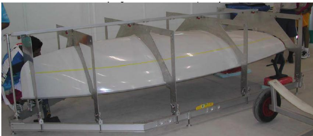
Figure H.1.4.10 The Europe hull inside the jig levelled and aligned using car jacks
