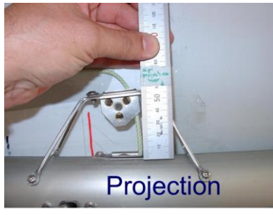
Spinnaker hoist height with the halyard at 90° to the spar.
